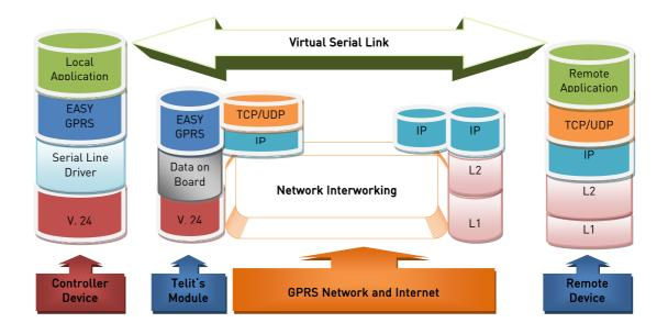
This particular implementation allows to the devices interfacing to the Telit GL868-DUAL module the use of the GPRS and Internet packet service without the need to have an internal TCP/IP stack since this function is embedded in the module.
